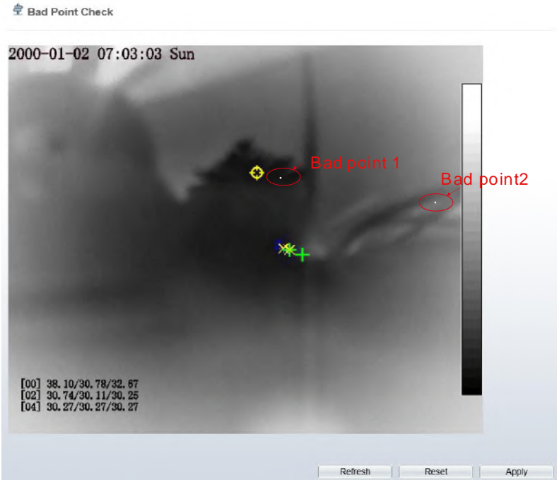
Figure 5-7 Bad Point Check
