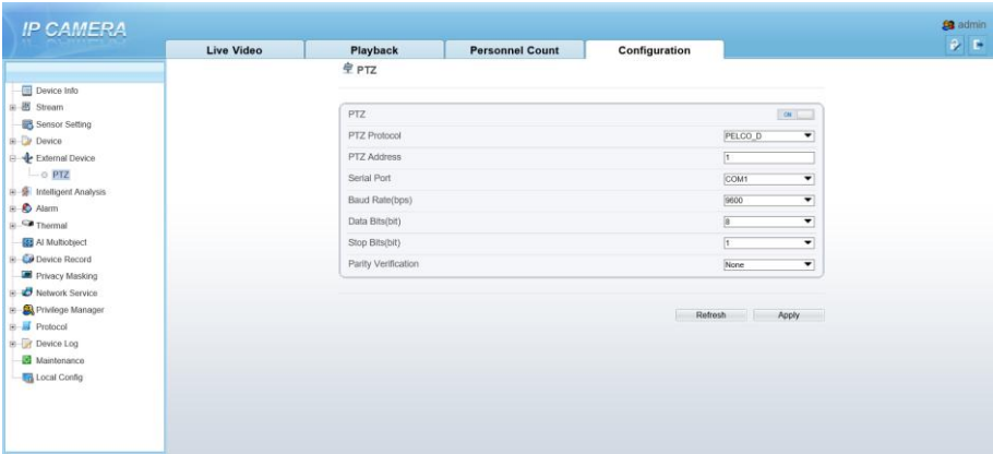
Figure 9-6 External device interface
